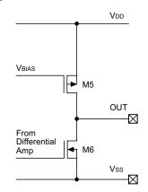
Because of the consideration for minimized power consumption, the max. output current is limited to about  $400\mu$ A for both source and sink drive. This is believed to be enough for most low power systems, however it is recommended to use the load resistor of >10k $\Omega$  for normal applications. In case of heavy load driving, an external buffer stage using bipolar transistors is recommended.
